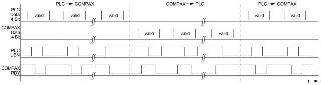
> It is important that the data ready message is only assigned after the data (when using PLC, one cycle later); i.e. once the data has been safely assigned.
